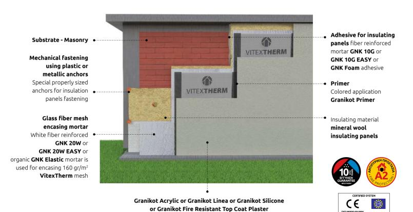
Colored top coats of acrylic or silicone based highly resistant to weather changes and to mechanical stresses
